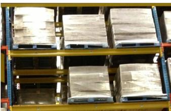
*Uniformly positioned and labeled pallets, one per location, are ideally suited to early drone scanning versions*
