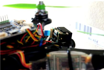
*Miniaturized barcode scanning engines are suitable payloads for scanning drones*
